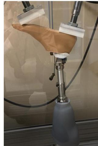
*Figure 1. 3D Printed Socket Being tested to ISO 10328 Ultimate Strength Requirements*
